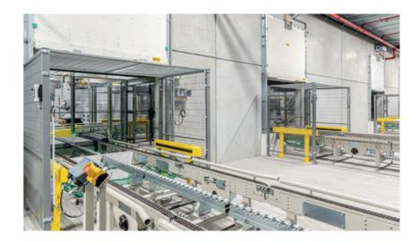
"With certified fireproof closures for conveyor belts, we are unique in Belgium. This is because these are subject to a different fire test standard than 'standard' fireproof gates."
