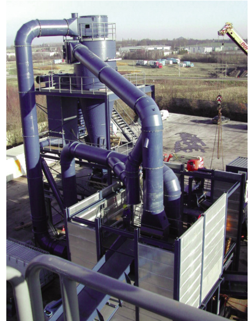
Light material separation subsequent to a 1400 HP-shredder
