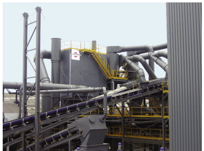
Shredder-light-fraction: sifter/extraction for 2 shredder lines
