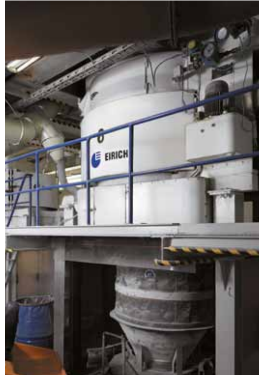
EIRICH mixer type R with 1,500 liters effective volume
