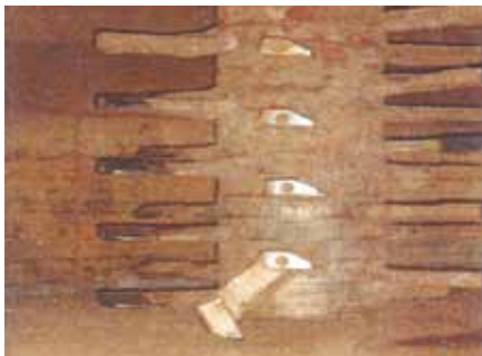
Interior view of an EIRICH sinter mixer Rotor after 3 months of operation
