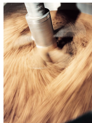
Fig. 2.1: Material current in the EIRICH intensive mixer
