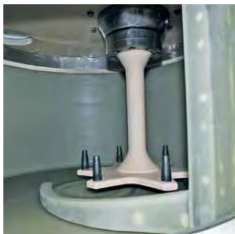
Mixer for contamination-free preparation Preparation of bioceramics in clean-room conditions
