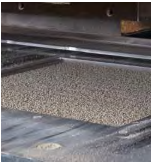
The good flow properties of the EcoPrep® granules enable uniform filling of the press mold
