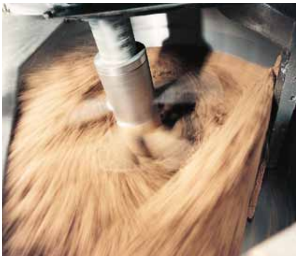
Material flow in the EIRICH mixer
