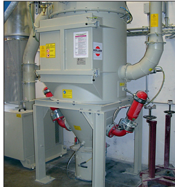
Round filter with container for extinguishing agent
