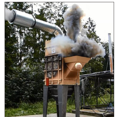
Explosion suppressed by ProPipePlus
