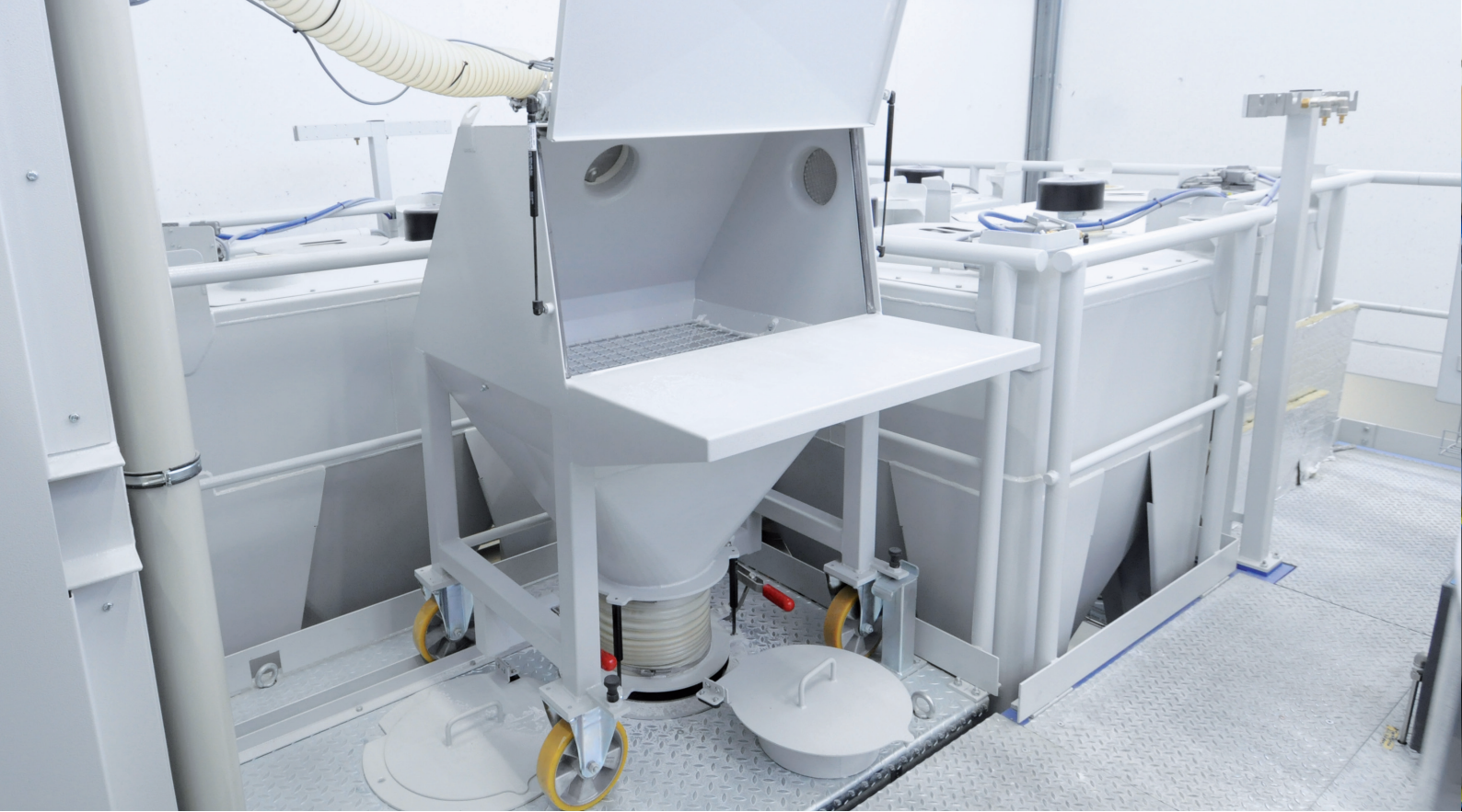
Sack chute type ST in mobile version for refilling dosages
