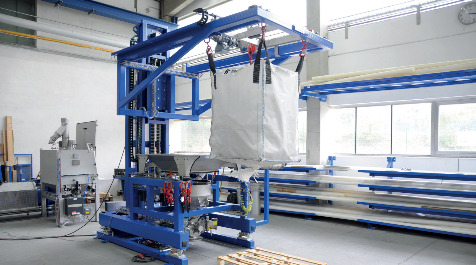
Big bag emptying station with movable support frame
