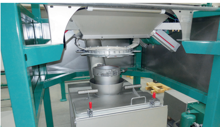
BE 1400 with sack chute and iris collar fastener
