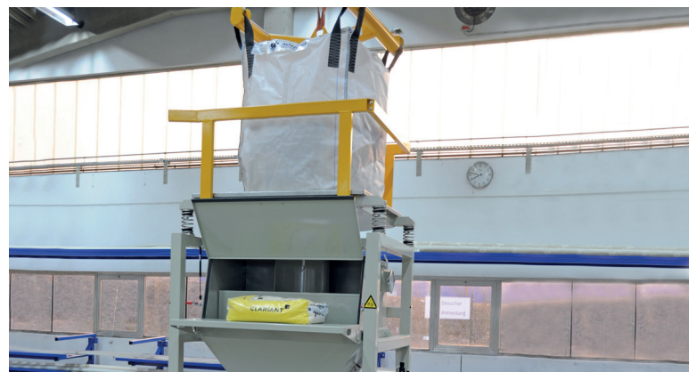
STBE with three-sided support railing
