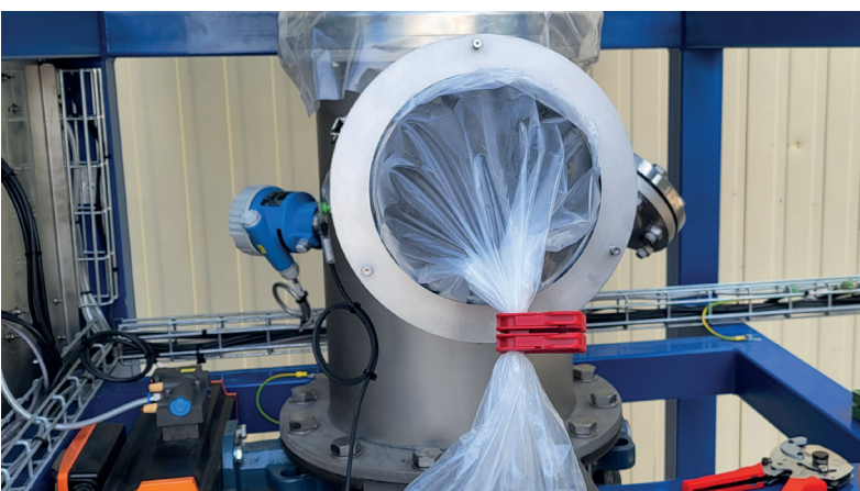
Docking system BE 2000 - foil tube with sealing clip
