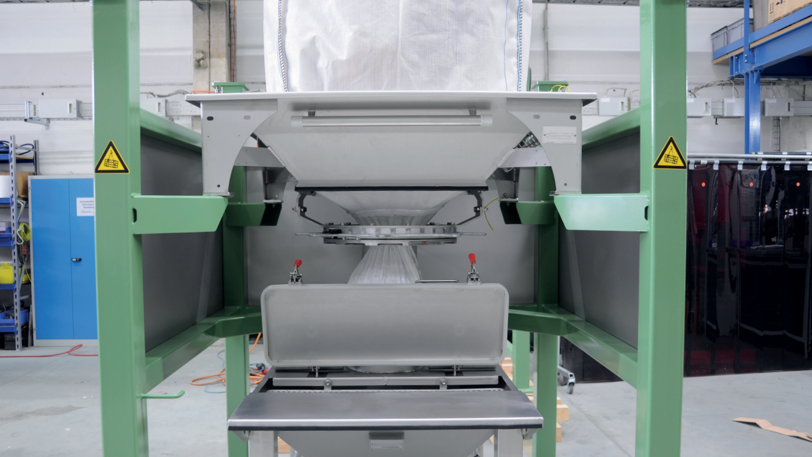
Combined sack/big bag emptier with iris collar closure for reclosing a big bag
