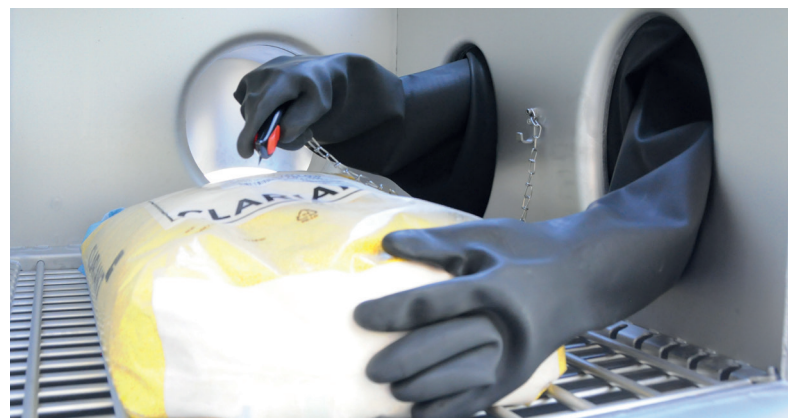
Sack handling via gauntlet gloves and safety knife
