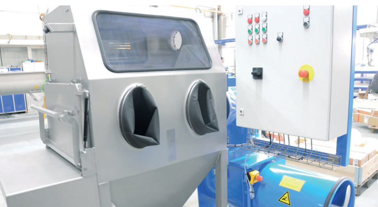
Input opening with tightly closing flap
