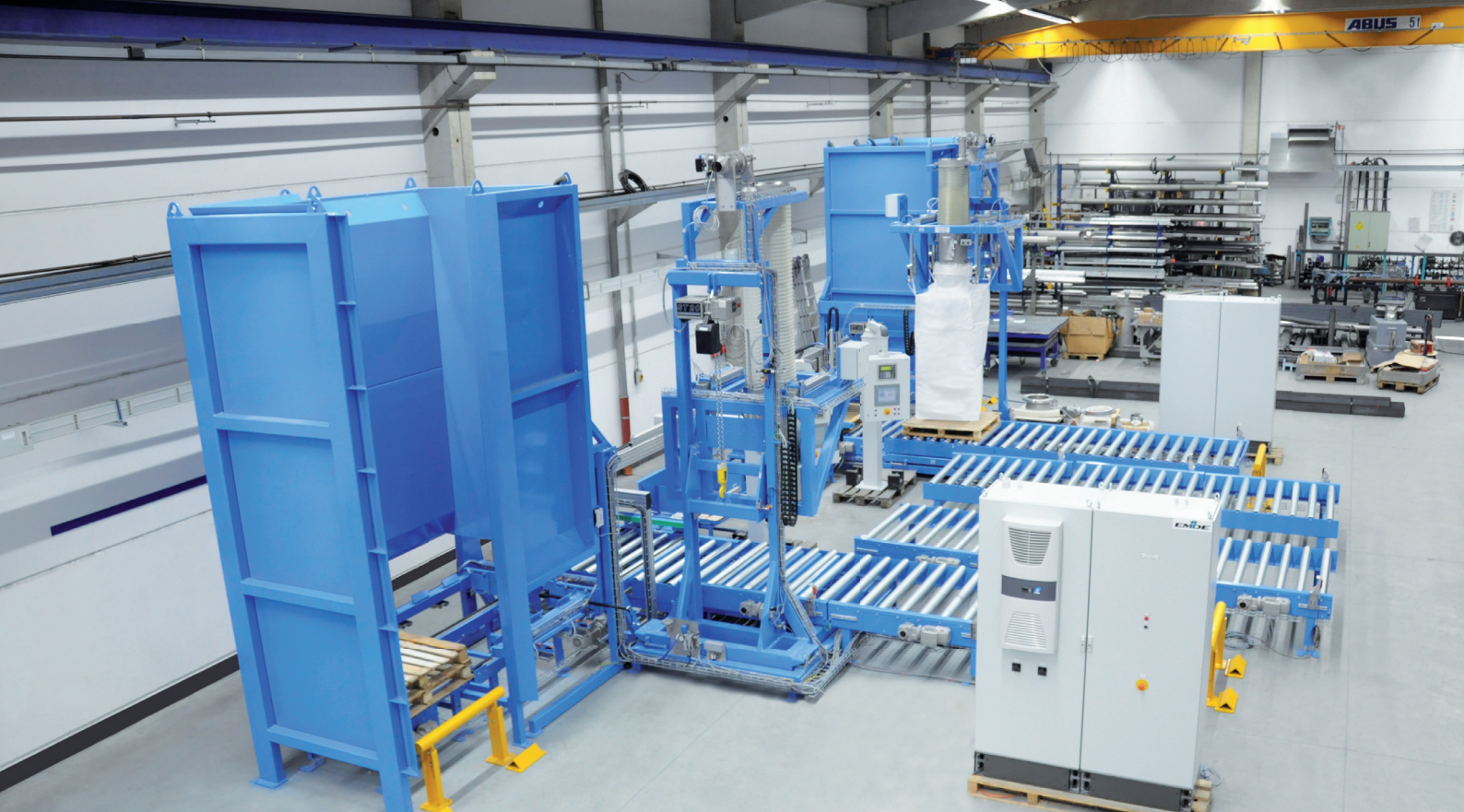
Dual filling system in final assembly for FAT test
