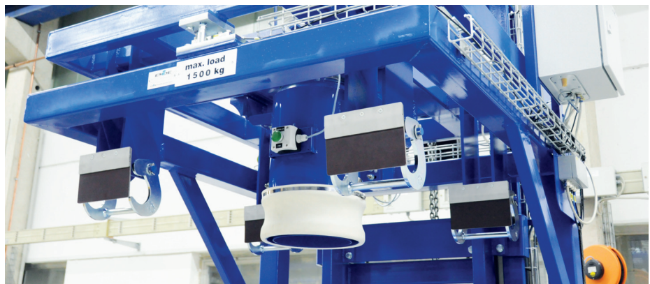
Swivel hook for Big Bag removal through fork lift prongs
