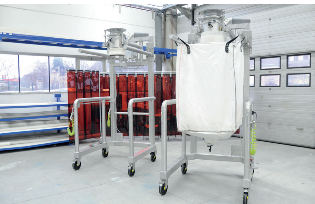
Mobile big Bag filling station with pipe forks
