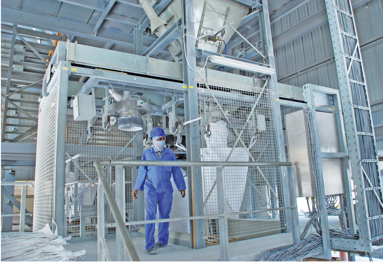
High performance filling system for up to 60 Big Bags per hour
