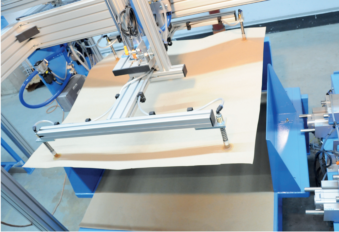
Paperboard sheet dispenser for moisture protection between pallet and Big Bag
