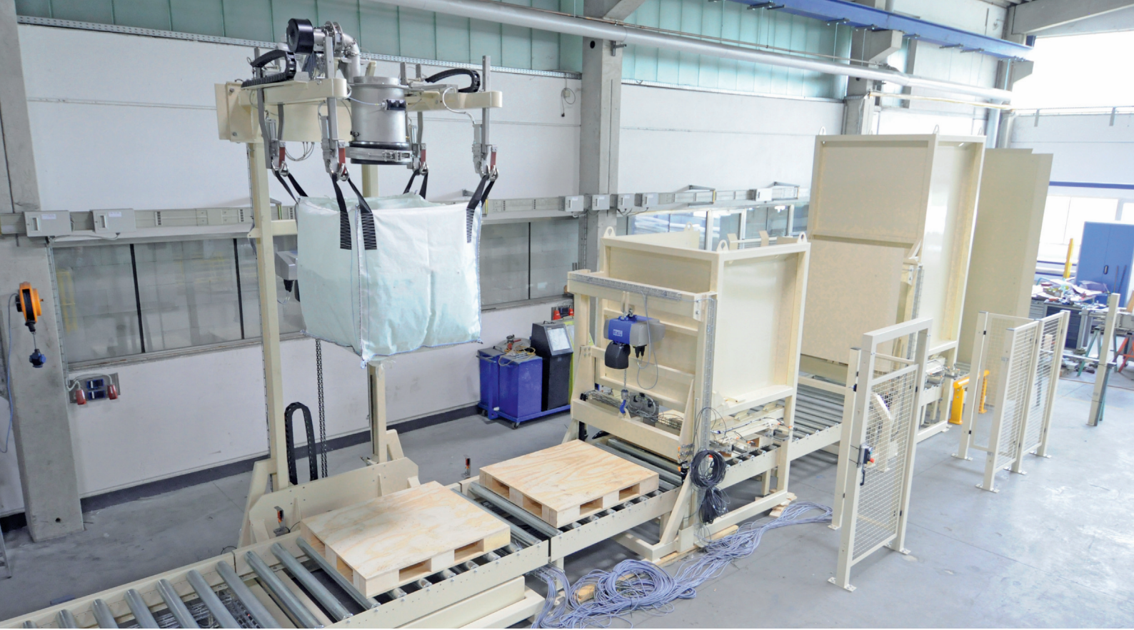
Big Bag filling system with release position for pallet stack and pallet magazine in final assembly
