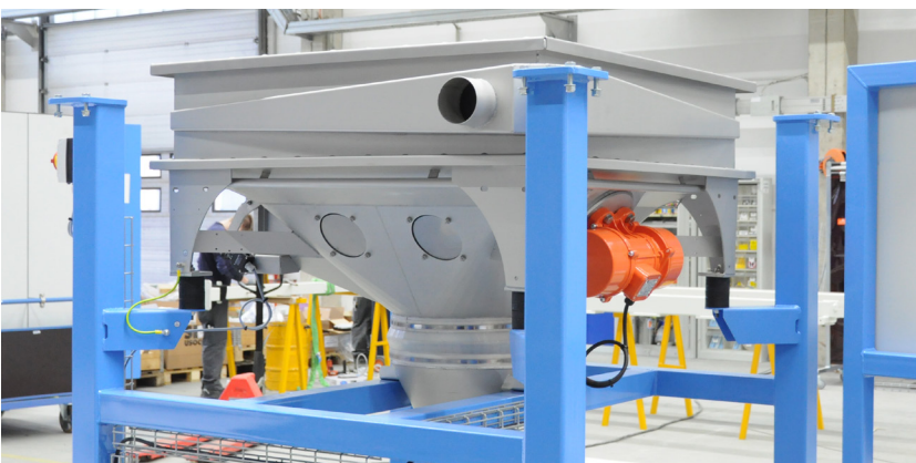
Type BE 1500 with dust aspiration duct
