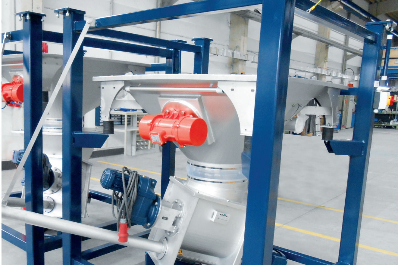
Big Bag emptying station with vibration discharge bottom and downstream metering screw
