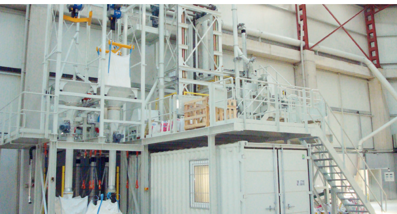
Big Bag emptying station in dosing system
