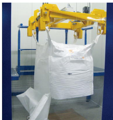
Big Bag bottom sliced open on 3 sides
