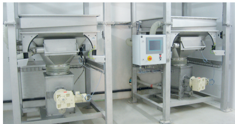
Big Bag emptying station with connected EMDE-LIFT
