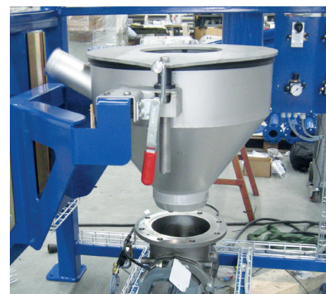
Docking plate with hand lever tighteners
