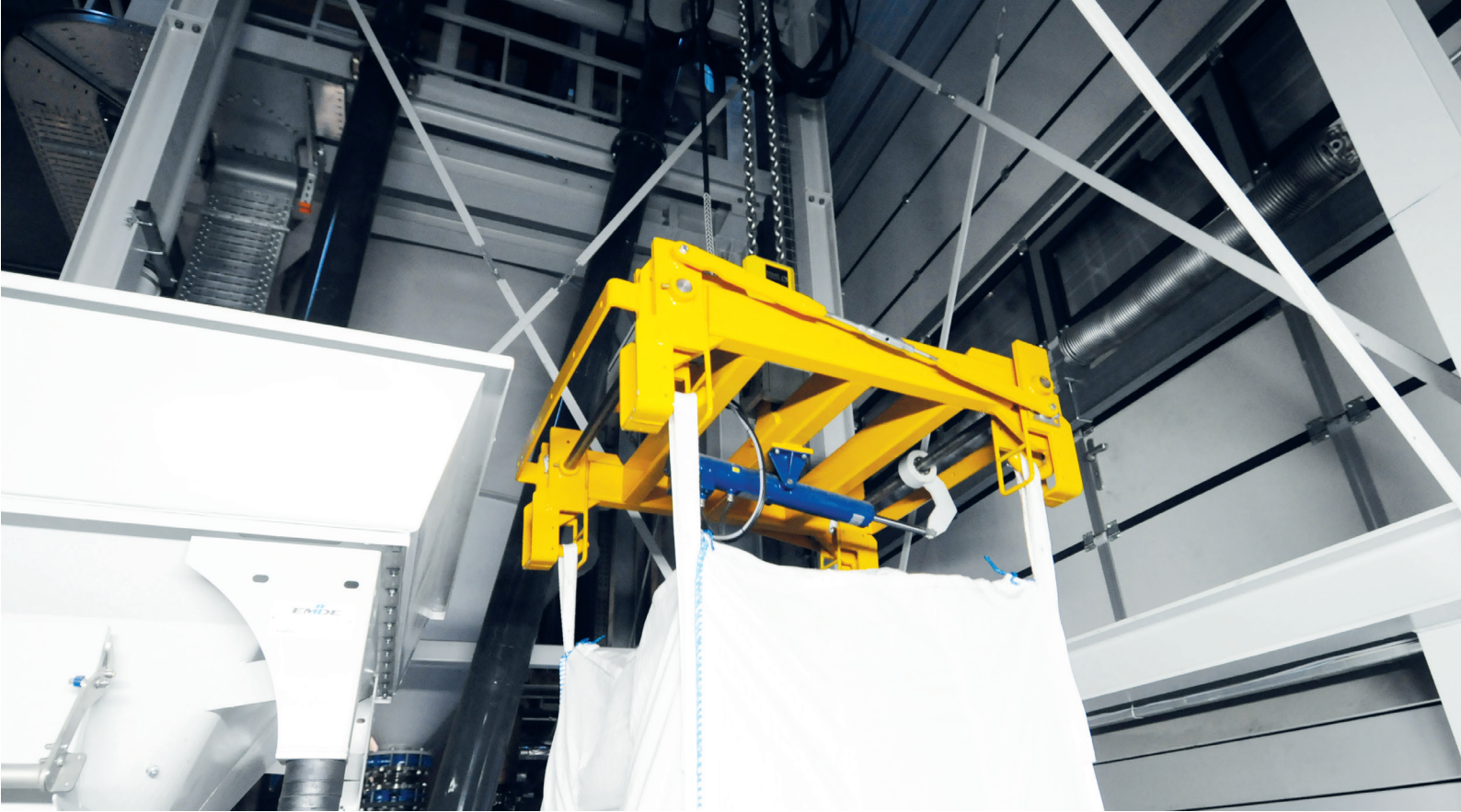
Special traverse with automatic loop release
