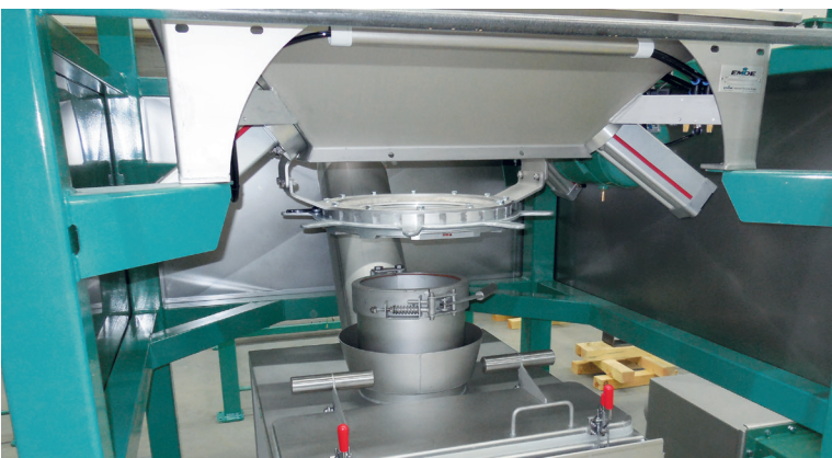
Type BE 1400 with discharge lock system
