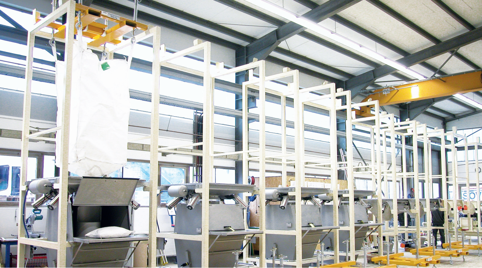
Combined bag/big bag emptying station in final assembly
