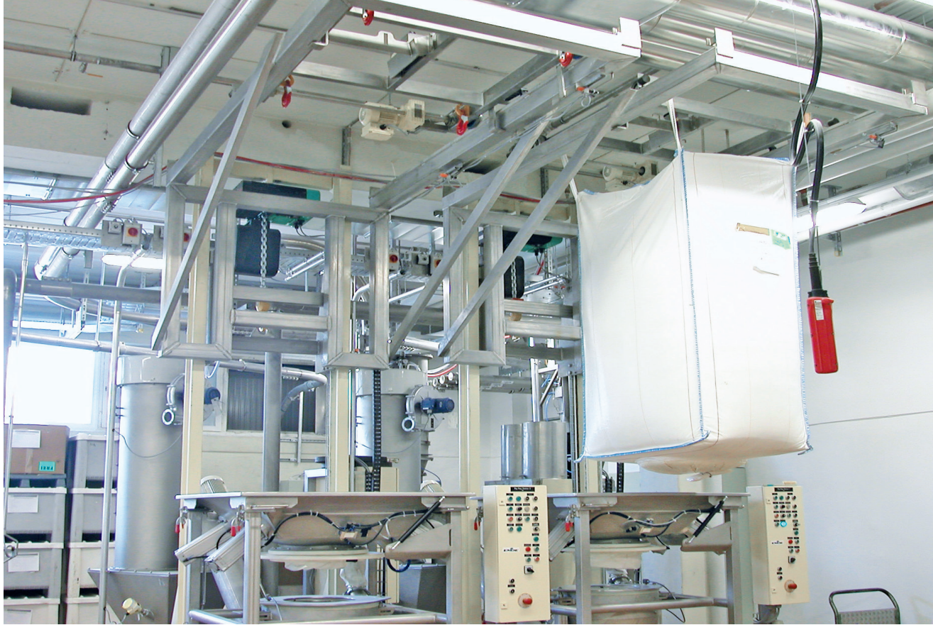
Big Bag emptying station with movable carrying frame
