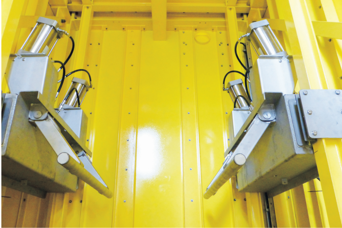
Side massaging device in Big Bag emptying system
